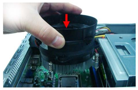
3. Secure the heat sink fan assembly to the screw holes on the main board using four screws.
